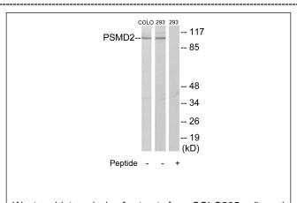
Western blot analysis of extracts from COLO205 cells and 293 cells, using PSMD2 antibody.
